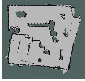
Figure 14: Generated Map with 0.3m/s Velocity throughout
