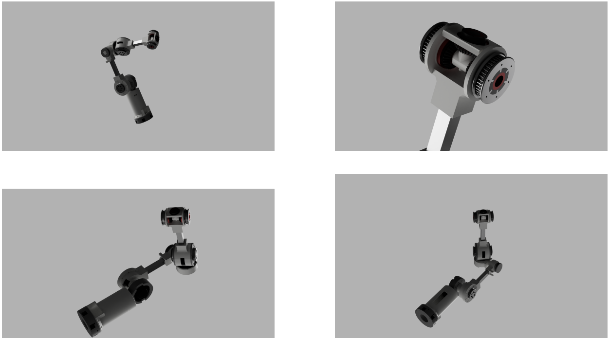
Figure 4-1: Final design: 3D CAD views from multiple angles showing actuator placement, elbow belt transmission, and the integrated wrist differential. This configuration balances weight reduction, mechanical simplicity, and dexterity, suitable for cinema-grade robotic motion.
