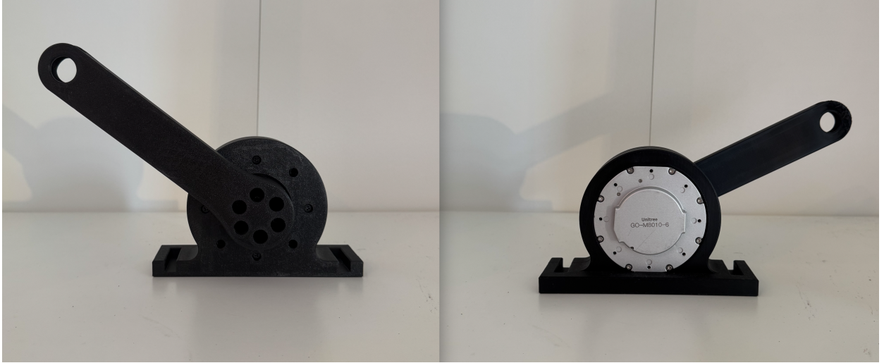
Figure 6-4: The repeatability test stand of the actuator.
