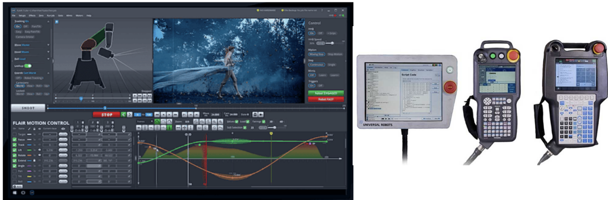
Figure 1-3: On the left shown the complex control software for key-framing the cinema robot arm, while on the right shown the outdated pendant-style controller that has been used in the industry for over two decades
