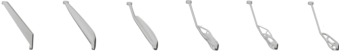
Figure 3. Generative design materials subtraction process
